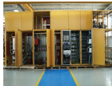
Simon Bolivar, Venezuela 805 MVA; large excitation system; highest voltage level, THYNE 6 solution
